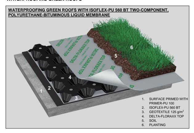
SOLUTION: Waterproofing green roofs with ISOFLEX-PU 560 BT, the two-component, polyurethane-bituminous liquid membrane.
