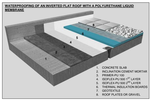
SOLUTION: Waterproofing of an inverted flat roof with a polyurethane liquid membrane
